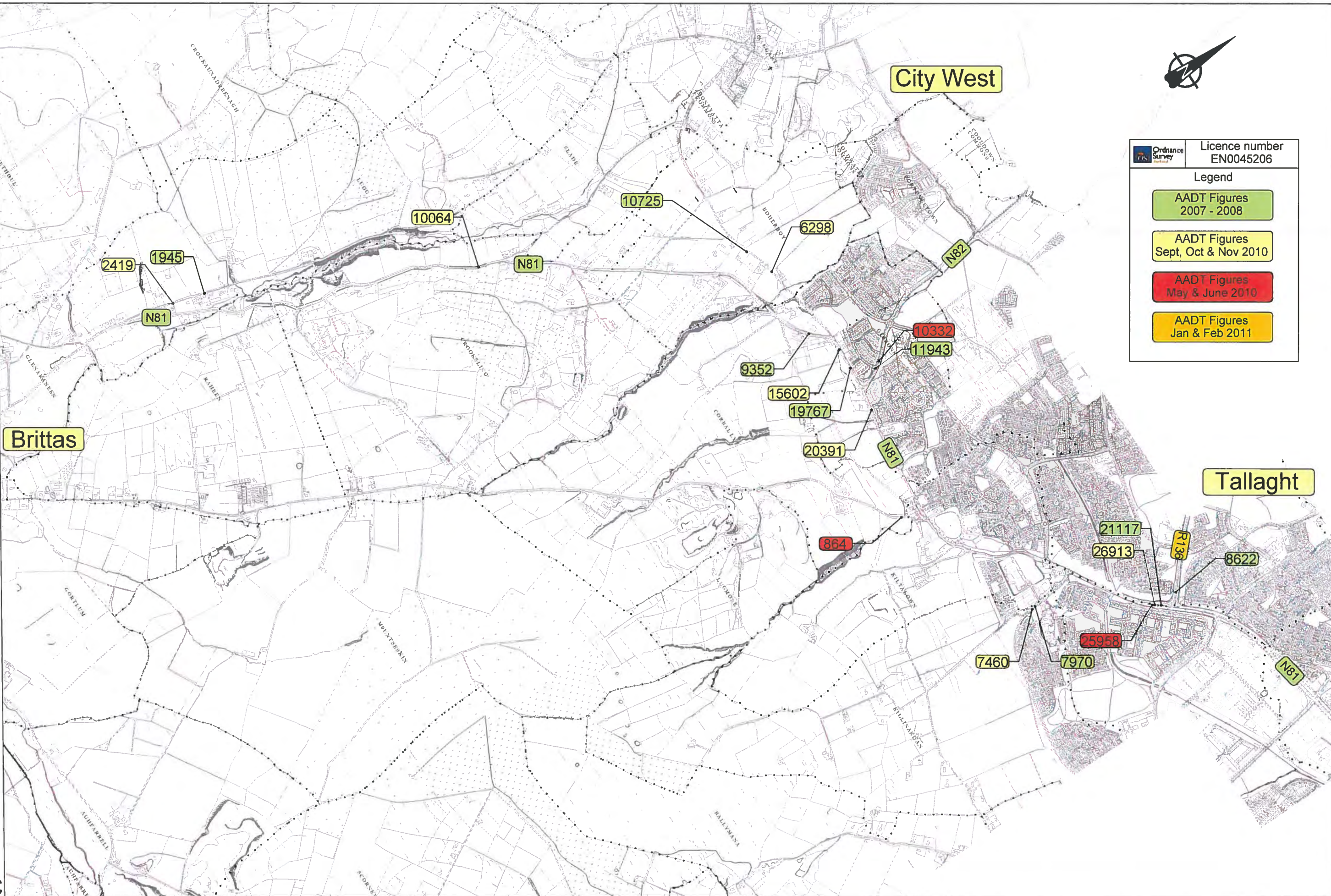
Figure 5.4 Existing A.A.D.T. Figures Sheet 4 of 4
